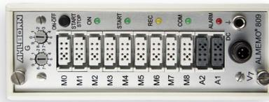
**Precision measuring instrument, latest V7 generation, nine measuring inputs
