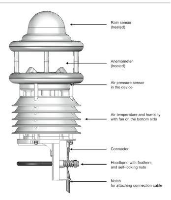
This measuring procedure is maintenance-free (no moving parts). For operation in winter the ultrasonic sensors can if so required be heated.
